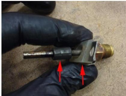
If the fuel nozzle has been bent, replace it. Even a slightly bent nozzle can restrict fuel flow into the burner, resulting in poor performance of the heater. Always be sure that the nozzle is clear and that the gaskets are in good condition. For further assistance, contact REE Technical Support.
