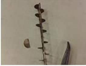
13. After removing the baffle, plug the tube with a wad of paper. This will maintain suction in the remaining tubes. Continue removing baffles
