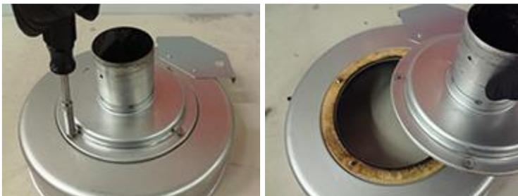
20. Clean the heat exchanger cover and muffler with Speedy White and allow to dry completely before reassembling the unit. You do not want the new gaskets getting wet.
