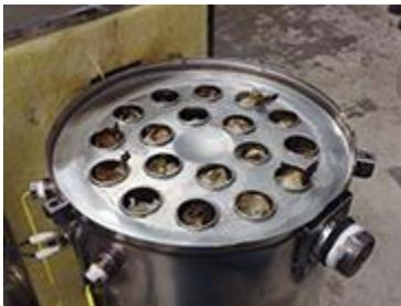
17. With the wire brush attached and your shop-vac still running, set the drill to the LOWEST SPEED, remove ONE paper plug, and insert the brush into the heat exchanger tube, brushing it until clean. Removing one paper plug at a time is a good way to prevent skipping a tube. Repeat this process for all remaining tubes. Using the low speed setting will lengthen the life of the brush and minimize the amount of carbon that is thrown into the air.
