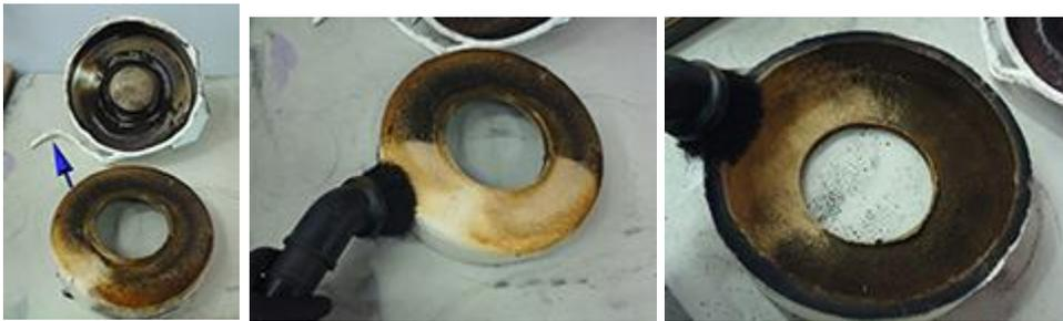
19. Remove the muffler from the heat exchanger cover. The muffler gasket should be replaced every time the heat exchanger is cleaned. (Part# 20476793)
