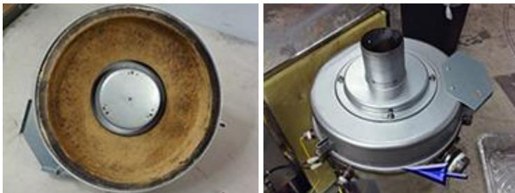
On the BS36UFF and the OM-148, the gap between the lip of the heat exchanger and the cover (indicated by arrow above) should be sealed with a high temperature (500 degrees F) silicone sealant.
