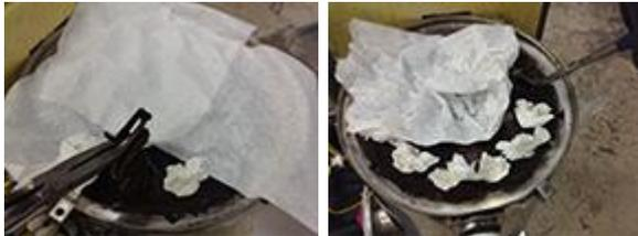
14. Spray the baffles with Speedy White (22oz. bottle Part# SW, or 1-gallon bottle Part# SW-GALLON) and rinse with hot water to remove soot buildup. Allow the baffles to dry completely before re-firing the unit.
