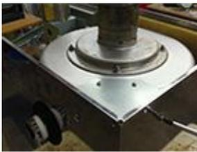
7. Remove the screws that attach the "L" shaped side and back panel, and remove the side/back panel.
