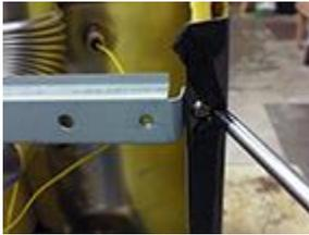
6. Remove (2) screws from heat exchanger bracket.
