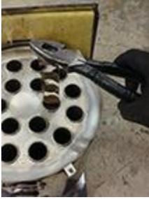
22. Install the new heat exchanger gasket. Notice that the cross section is rectangle shaped. The gasket should lay flat, as pictured below.
