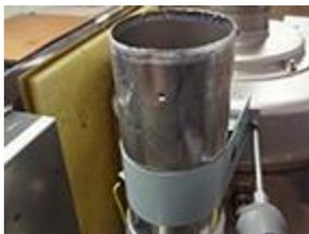
9. Remove the three screws/8mm nuts that attach the heat exchanger cover. In some models, the gap around this cover may be sealed with a high-temperature silicone. Use a utility knife to cut the silicone, allowing the cover to be removed.
