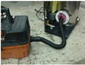
11. Remove the heat exchanger cover. Be careful to avoid damaging the insulator (also known as the insulation bonnet, inside the heat exchanger cover).
