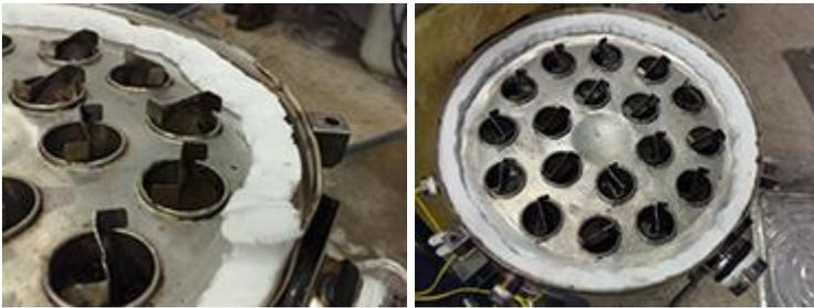
23. Put the heat exchanger cover and muffler back together, using a new muffler gasket. The muffler will only go back on one way, with the seam of the exhaust toward the back of the unit. Place the insulator back into the cover. Flip the cover right-side up, line up the screw holes, and gently place the cover/insulator back in place on top of the heat exchanger. Replace and tighten the screws/nuts that hold the cover down.
