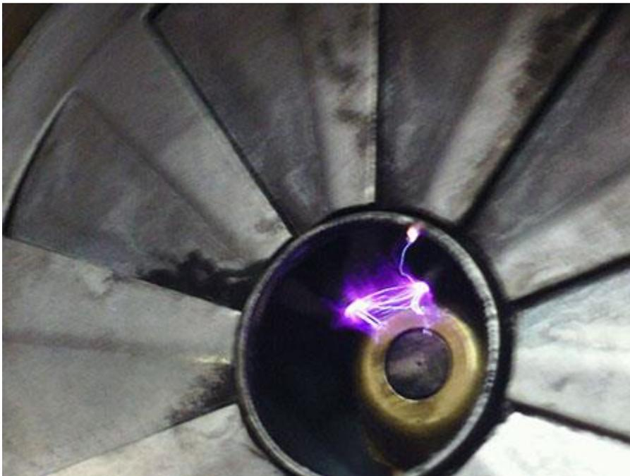
20. Reinstall the burner assembly. Be careful not to pinch any of the wires between the burner assembly and heat exchanger.
