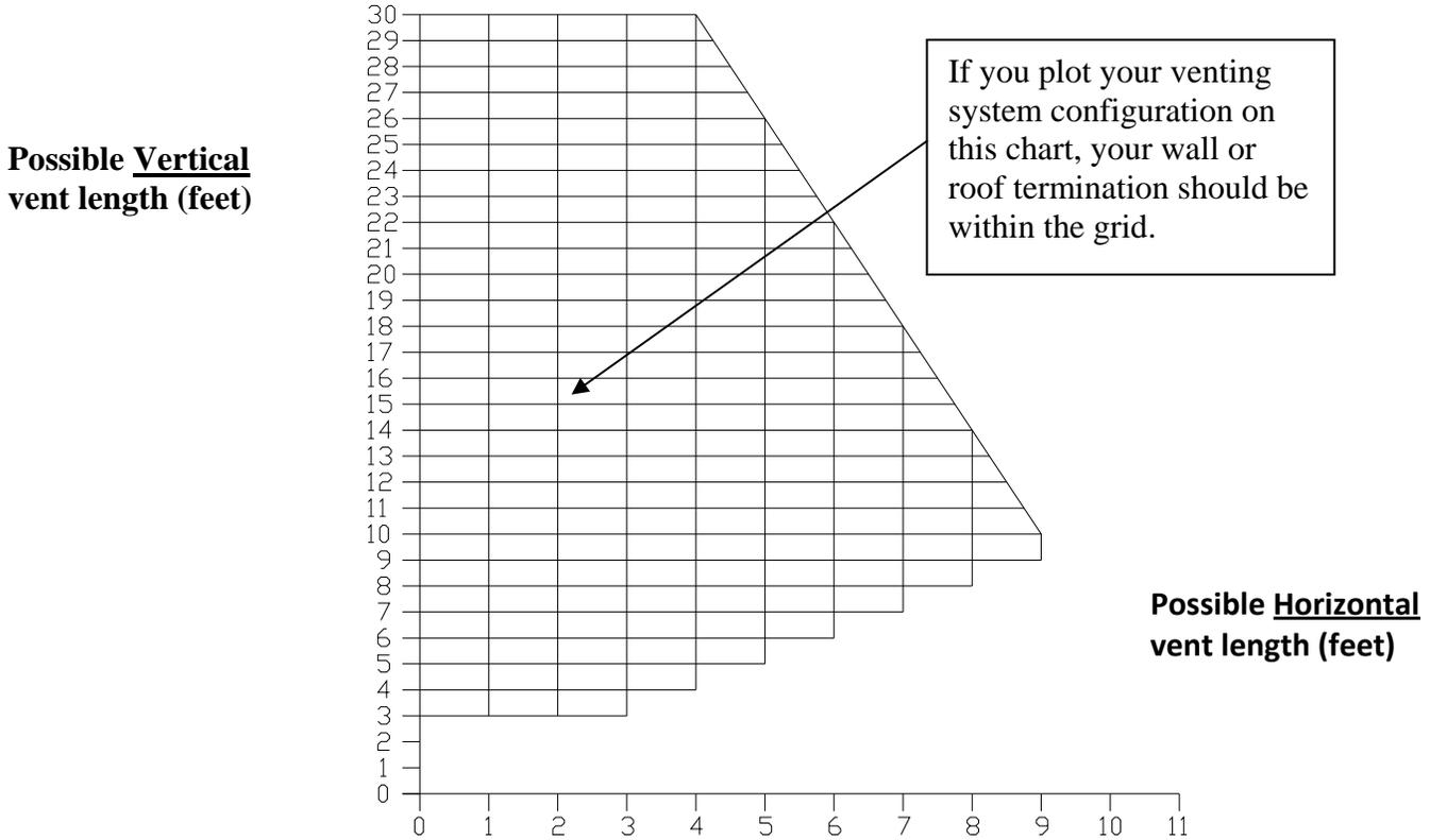
Let's imagine an installation consisting of a horizontal vent coming out at the back of the stove on a total distance of 8 feet. This horizontal run is followed by a Tee and a 6-foot vertical rise. This type installation is not acceptable. As you can see, the vent termination is clearly outside the allowed configuration zone on the chart. The venting system does not have at least one foot of vertical rise for each foot of horizontal run.
